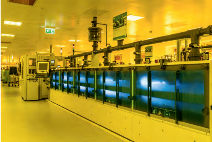
Etching technology process of ISA-PLAN® resistors
